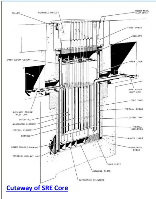
The U.S. Department of Energy (DOE) describes the incident that occurred at SSFL's Sodium Reactor Experiment (SRE) during a two week period in July 1959 as a core damage accident. At that time the SRE, a small federally funded research reactor located in the Simi Hills about 30 miles northwest of downtown Los Angeles, suffered significant fuel damage as a result of overheating
