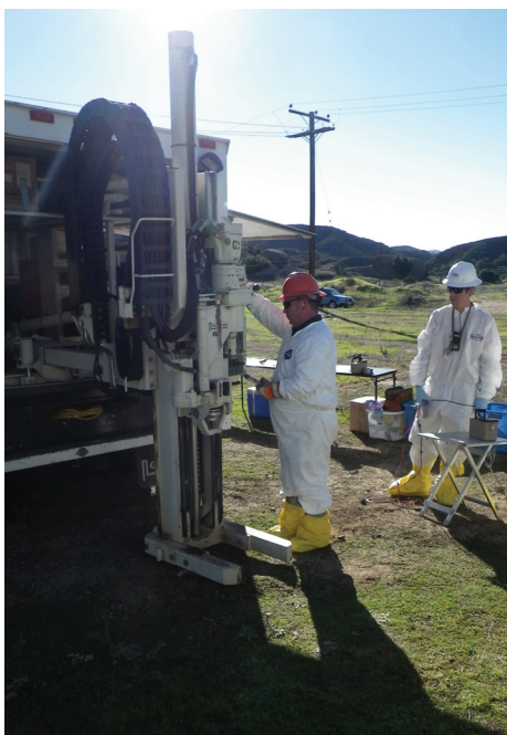
Figure 2: Workers conducting subsurface soil sampling in Area IV with a direct push drill rig
